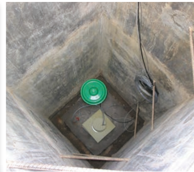
AfricaArray seismic stations in Dodoma, Tanzania (top left) and Zomba, Malawi (top right and bottom). Top right photo was taken looking down into the 3-m deep seismic vault shown in photo at left at the Geological Survey in Zomba, Malawi. Top left photo was taken looking down into the 4-m deep vault at the Geological Survey in Dodoma, Tanzania. Photos credit: Andy Nyblade.
