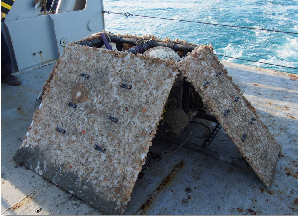
Figure 3. The shallow trawl-resistant absolute pressure gauges were covered in mud and marine life and had to be completely cleaned before returning to shore. Photo credit: Erin K. Todd
