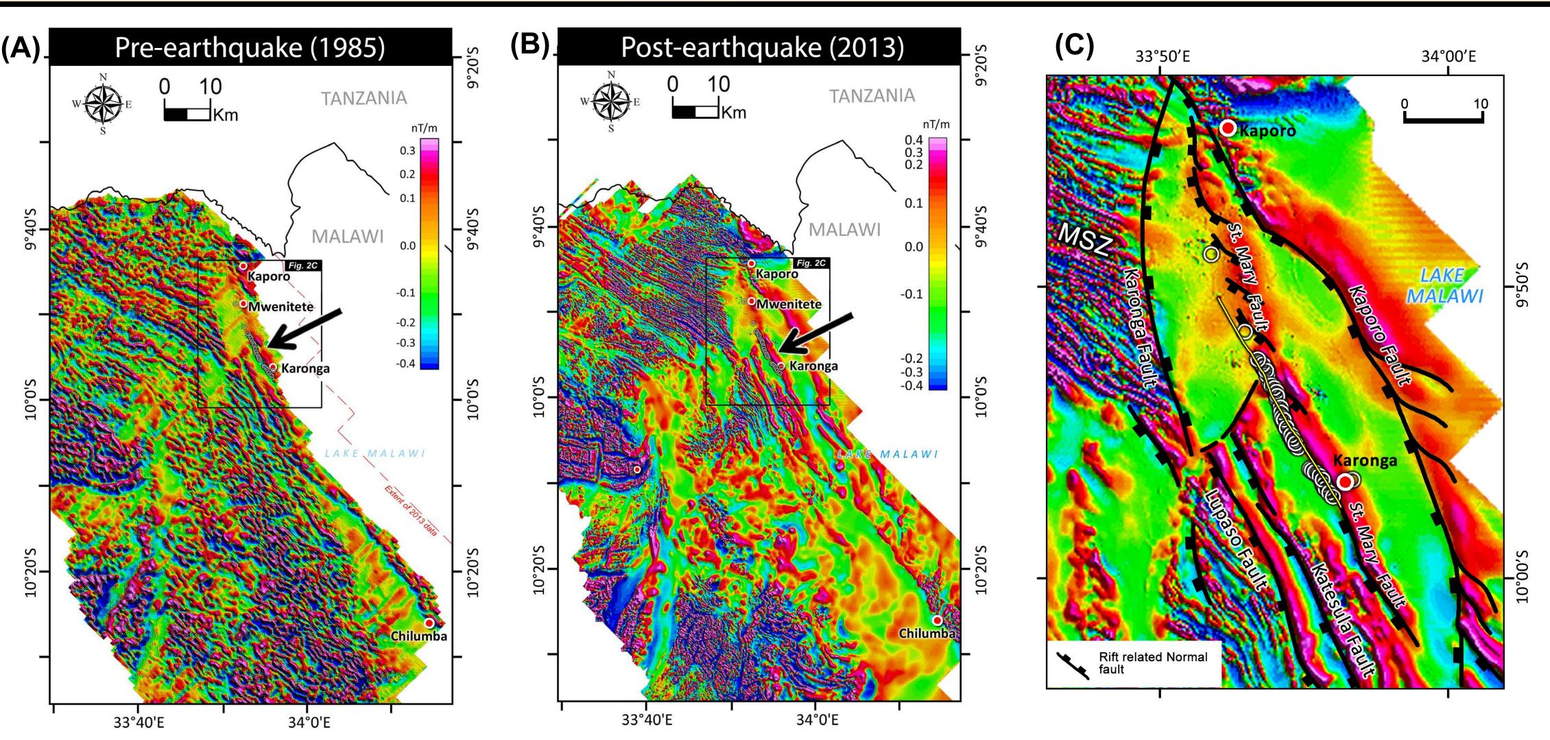
Fig. 2 (A-B) First vertical derivatives (Dz) of the RTP pre- and post- earthquake aeromagnetic grids of NW Malawi, overlaid with earthquake surface rupture locations (white circles). Black arrow points at prominent magnetic lineament. (C) The 2013 aeromagnetic grid showing interpreted buried basement-rooted faults. Yellow line represents InSAR fault model by [1] and [2].
