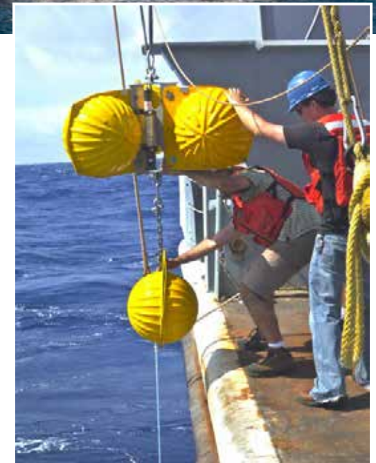
Deploying moored hydrophones near the Mariana Trench axis
