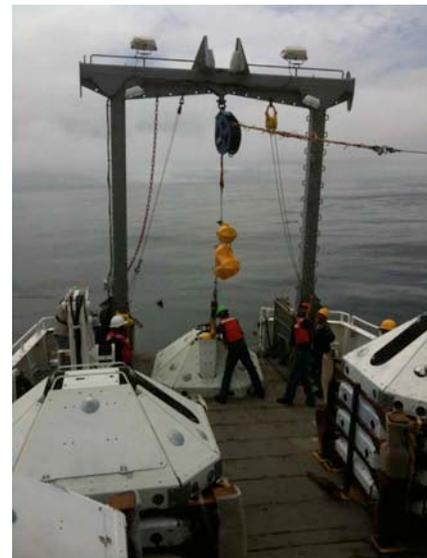
Figure 3. New trawl-resistant OBS's being deployed off Cascadia. From July, 2011 cruise report (Tolstoy, Trehu). <http://pages.uoregon.edu/drt/CIET/doku.php>
