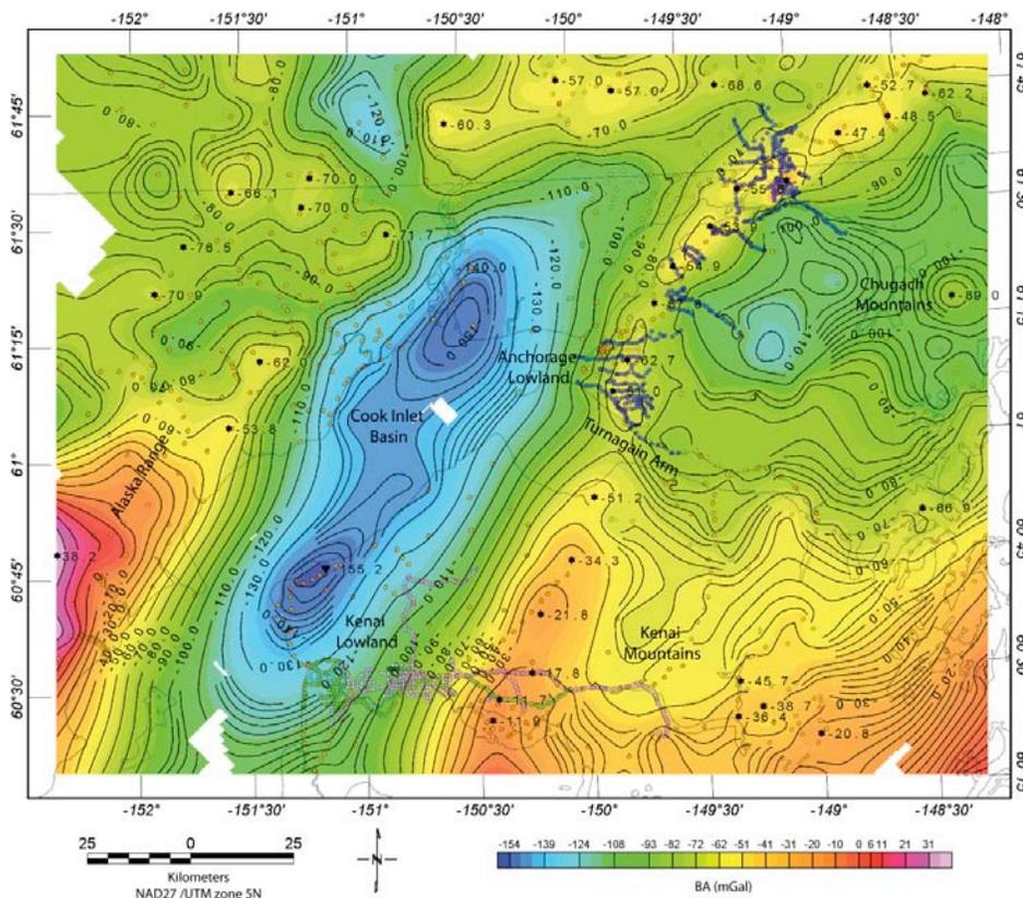
Figure 1 – Simple Bouguer anomaly map (with reducing density of 2670 kg/m<sup>3</sup>). Gravity points were compiled from pre-1996 existing data, 2009 (pink and green points) and 2010 (blue points). A survey completed in mid-August 2011 collected ~400 new gravity readings in a region from 61.4 to 61.75°N and 148.7 to 150°W.
