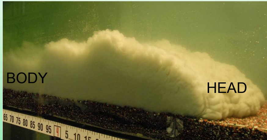
Sequeiros/Hybrid saline/turbidity current over mobile bed vtchl.illinois.edu
