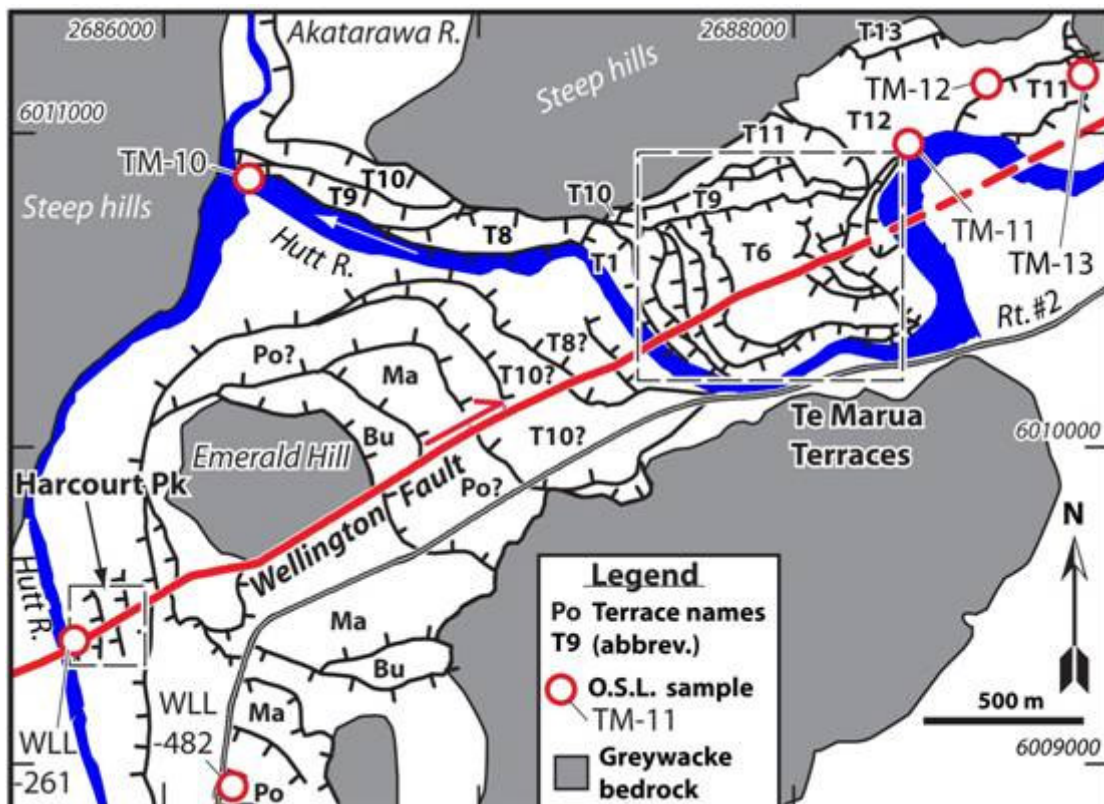
Figure 8.1. Wellington Fault through the Harcourt Park, Emerald Hill and Te Marua Terraces area (after Berryman 1990, modified by Little et al manuscript in prep.). Terrace names: Po, Porewa; Ma, Marton; Bu, Burnand. Dashed-box around Te Marua Terraces area denotes location of Figure 8.2 and approximate location of Figure 8.3.
