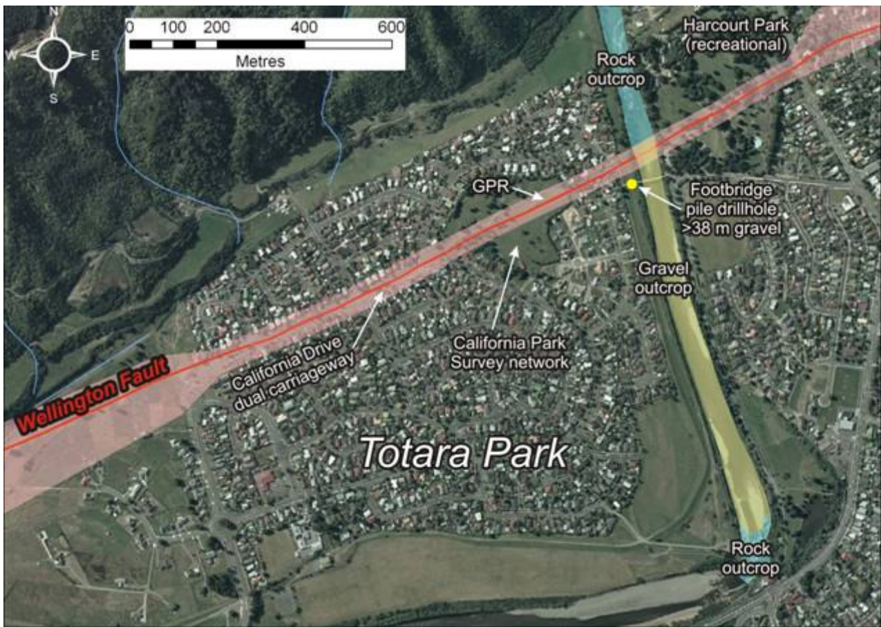
Figure 7.2. The location of the trace of the Wellington Fault at Totara Park is tightly constrained, as indicated by the narrowness of the Avoidance Zone defined by Van Dissen et al. (2005). At either end of the trace, the location of the fault is less well-known, and the width of the Fault Avoidance Zone is consequently substantially broader.
