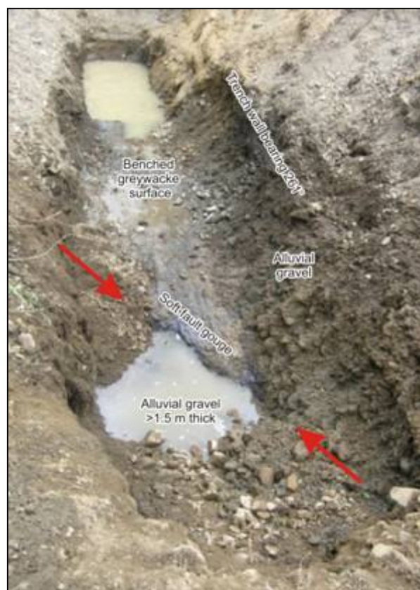
Figure 5.2. The Manor Park trench exposure of the Wellington Fault, showing the bench cut on sheared greywacke rock and lithified gouge, soft gouge near the lip of the surface, and unfaulted alluvial gravel overlying the bench. Note the obliquity between the trench wall and the strike of the fault (strike ca 44^\circ ).
