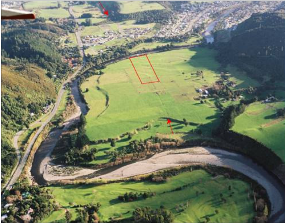
Figure 8.3. Oblique aerial view to the SW along the Wellington Fault (arrowed) at Te Marua. The Hutt River winds through this area and has left behind a flight of abandoned river terraces, which are progressively dextrally displaced by the fault. Box shows area of Figures 8.5b & 8.6a. Photo: D.L. Homer.
