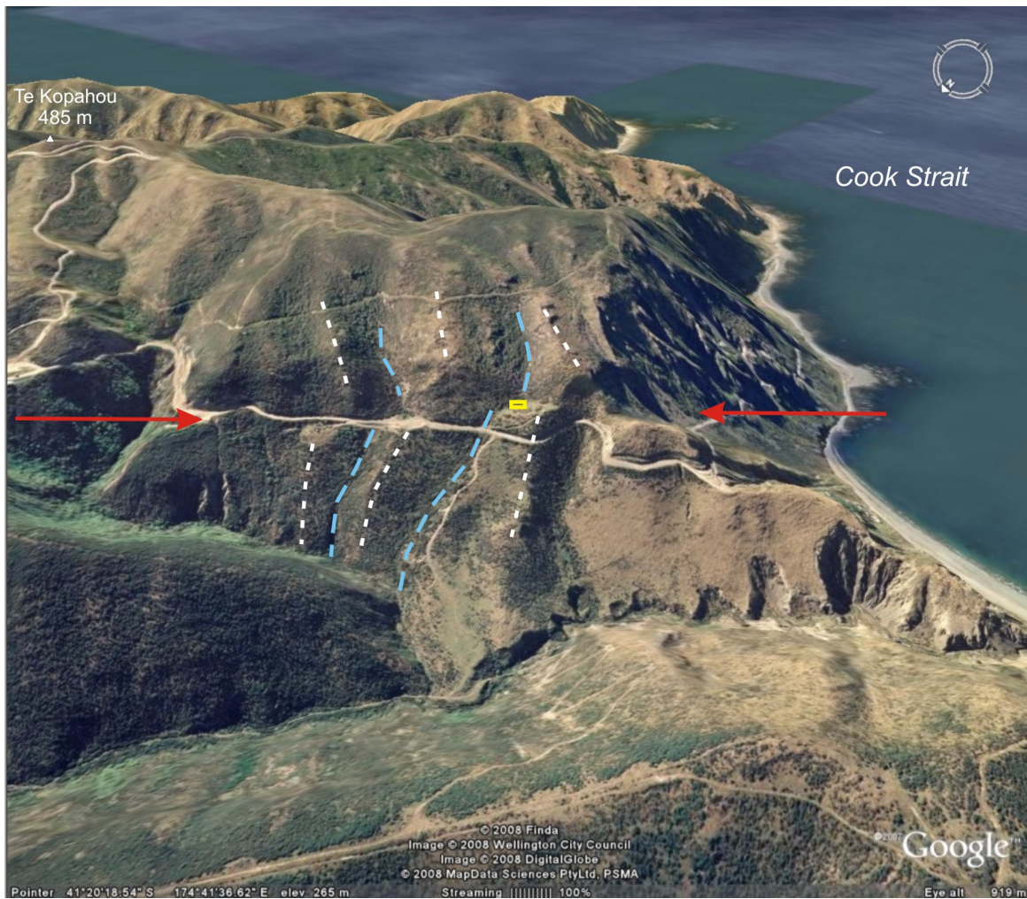
Figure 1.1. Oblique aerial view of the Wellington Fault above Cook Strait. The ca 042°-striking fault trace is marked by red arrows. White lines mark ridgelines (spurs), while blue lines mark adjacent streams. The Te Kopahou trenches (yellow box) were sited behind a prominent shutter ridge (offset spur). Image from Google Earth.
