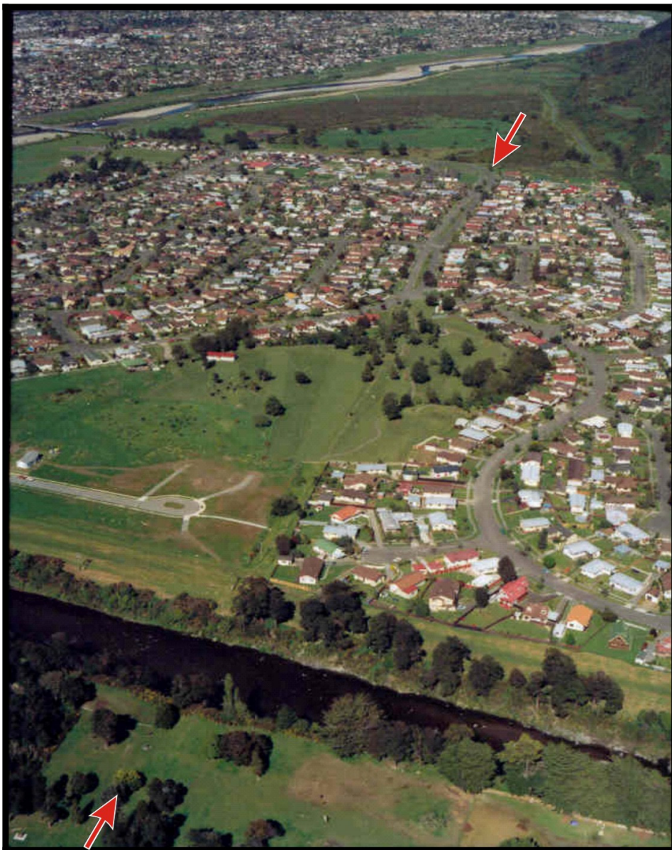
Figure 3.1. The location of the Wellington Fault (between arrows) at Totara Park was known before development of the subdivision. Note the dual carriageway of California Drive with houses on each side set back from the fault. California Park, a recreational reserve (also Figs. 3.2 & 3.3), is also used to mitigate rupture hazard. In the foreground on the northern side of the river, preservation of the Wellington Fault scarp was one of the wishes of the person who donated Harcourt Park to Upper Hutt City Council.
