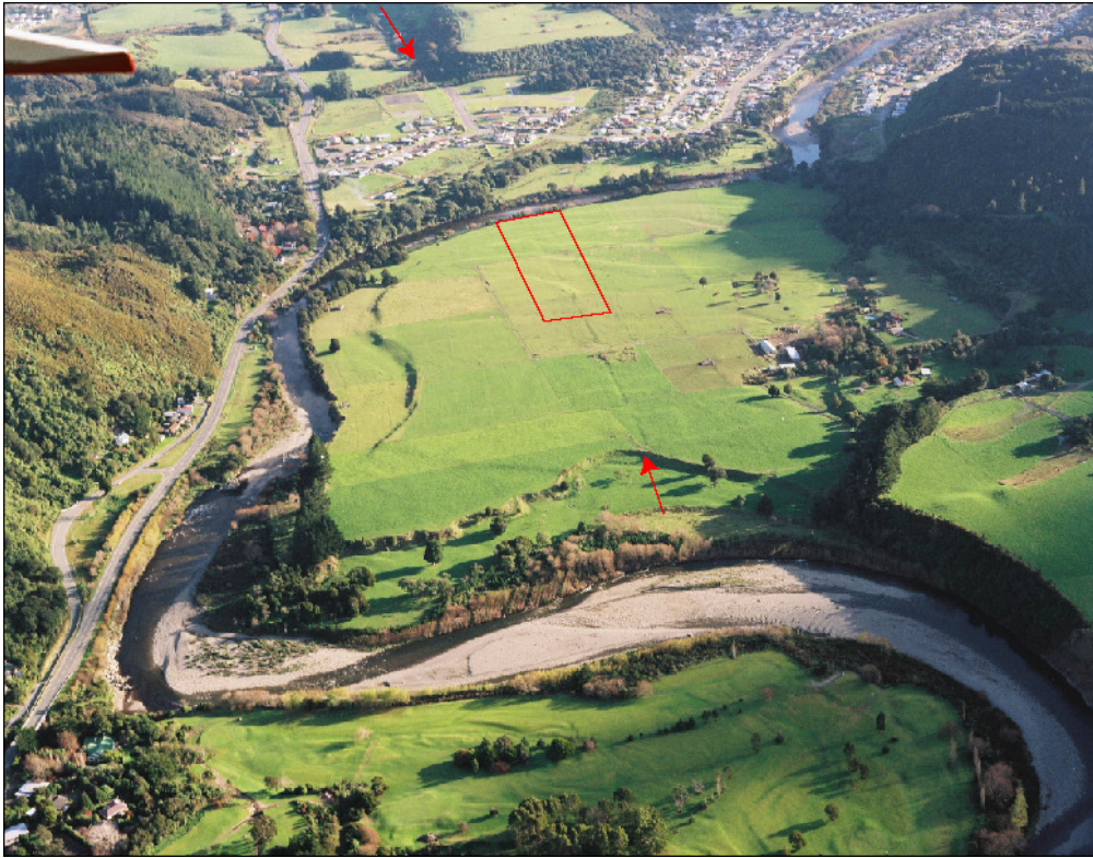
Figure 4.5. Oblique aerial view to the SW along the Wellington Fault (arrowed) at Te Marua. The Hutt River winds through this area and has left behind a flight of abandoned river terraces, which are progressively dextrally displaced by the fault. Box shows area of Figures 4.7b & 4.8a. Photo: D.L. Homer.
