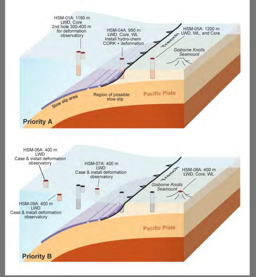
Phase 1: Seven shallow (~400-1200 m below the seafloor) riserless sites to collect samples and geophysical logs of the overriding and subducting plates, and install observatory equipment to monitor nearsurface changes in deformation, seismicity and physical properties throughout a SSE cycle and characterize the distribution of SSE slip with very high fidelity.
