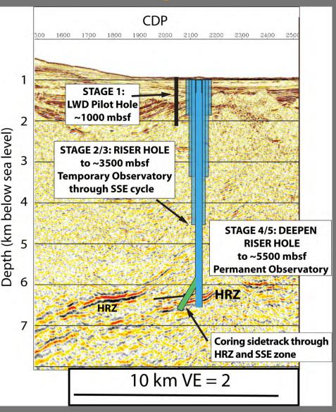
**Phase 2:** A deep riser hole (~5-6 km below the sea floor) to penetrate the subduction interface and *directly sample rocks from the SSE source region*, collect logs across the fault zone(s), and measure temperature, fluid pressure and chemistry, and stress.
