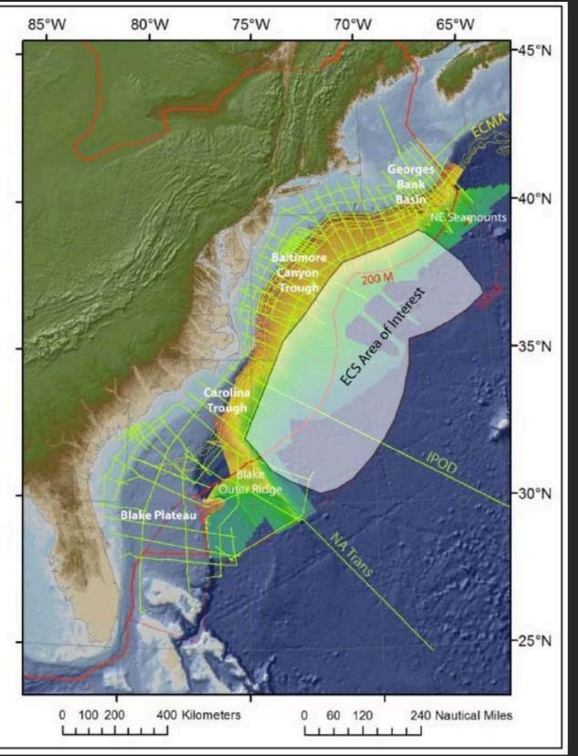
Task: Acquire multibeam bathymetry (led by NOAA and UNH) and multichannel seismic reflection and refraction data (led by USGS)
